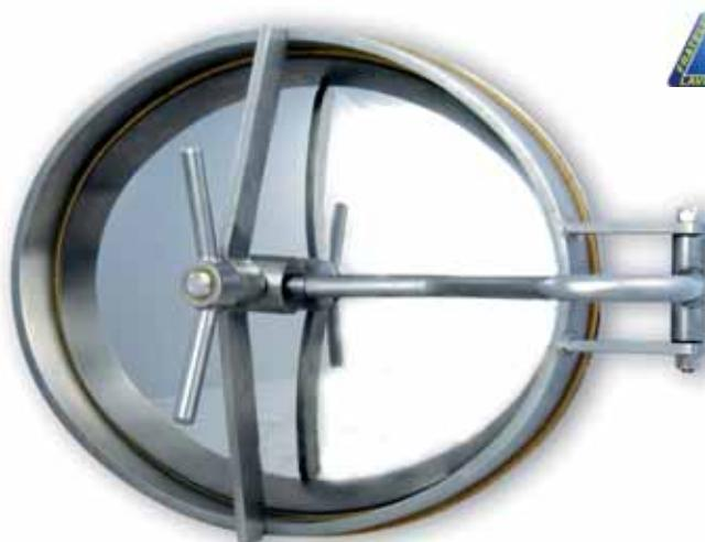
Oval shaped manhole door type "milk" in AISI 304 or AISI 316/L stainless steel - inward opening it is possible that the cover comes out frame fabricated in flat stainless steel - 60x12 access 520 x 420 mm.
