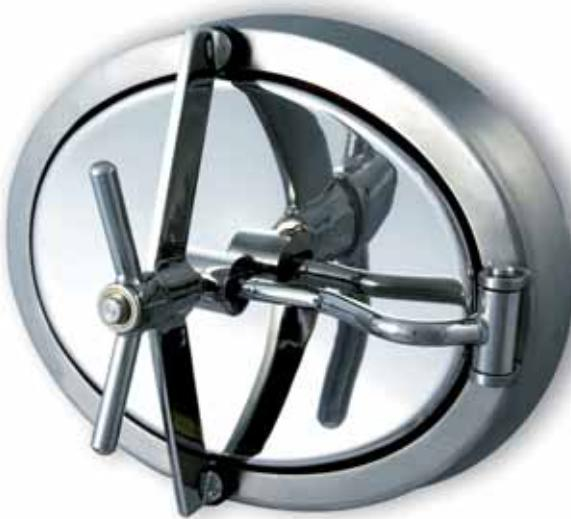
Oval shaped manhole door in AISI 304 or AISI 316/L stainless steel - inward opening it is possible that the cover comes out frame fabricated in flat stainless steel - 30x12 H mm. 80x5 access 440 x 340 mm. Certifications: PED
