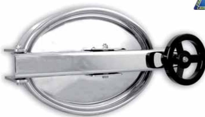
Oval shaped manhole door in AISI 304 or AISI 316 stainless steel - outward opening - frame fabricated in flat stainless steel - access 440 x 310 mm.
