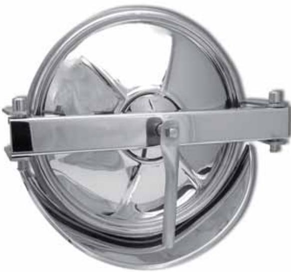
Circular manhole door in AISI 304 or AISI 316 stainless steel - light-duty - frame fabricated in pressed stainless steel sheet - access 300 - 420 mm.
