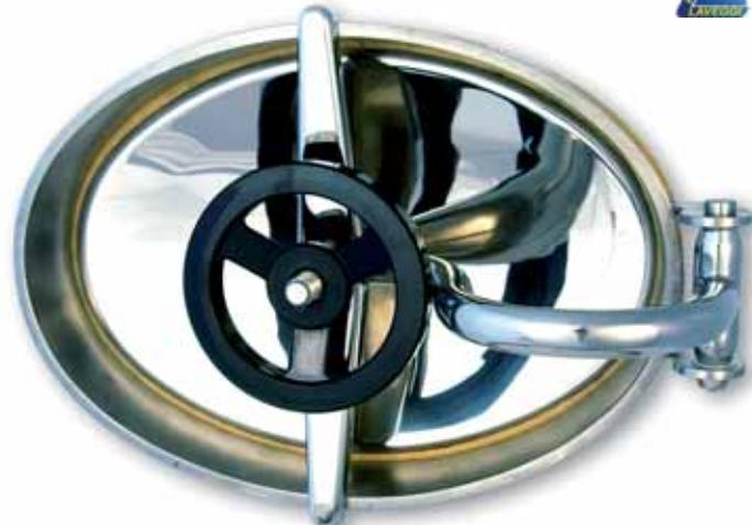
**Oval shaped manhole door type "export" in AISI 304 or AISI 316 frame fabricated in flat stainless steel - inward opening it is possible that the cover comes out with support arm - access 440 x 310 mm.**
