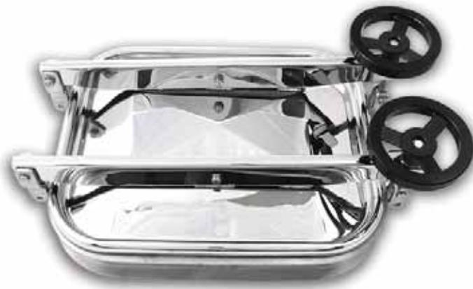
Rectangular manhole door for winemakers, in AISI 304 or AISI 316 stainless steel - frame in flat stainless steel or iron - horizontal outward opening - access 530 x 410 mm.
