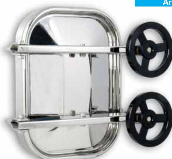
Rectangular manhole door in AISI 304 or AISI 316 - stainless steel - frame fabricated in flat stainless steel - outward opening - access 420 x 310 mm.
