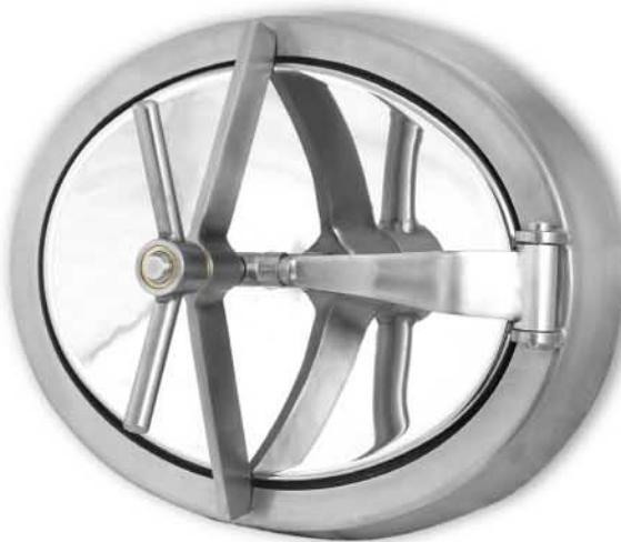
Oval shaped manhole door type "fruit juice" in AISI 304 or AISI 316 stainless steel - inward opening - frame fabricated in flat stainless steel 30 x 12 mm. H 80x3 mm. - access 440 x 340 mm.
