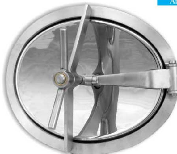
Oval shaped manhole door type "fruit juice" in AISI 304 or AISI 316 stainless steel - inward opening - frame fabricated in flat stainless steel 30 x 12 mm. - access 440 x 340 mm. (available on request bending for various vat diameters).
