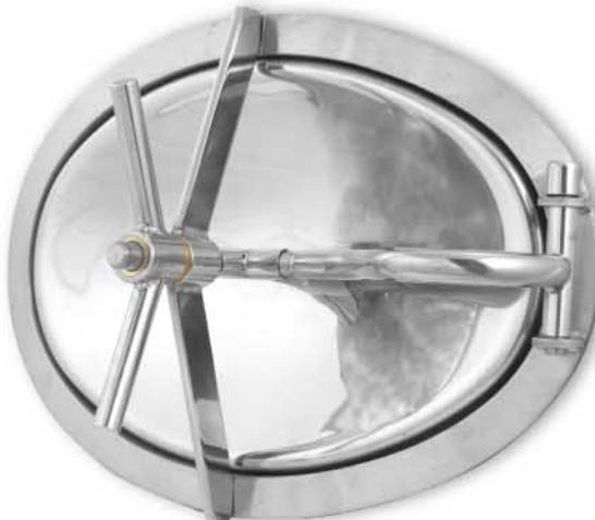
Oval shaped manhole door type "fruit juice" in AISI 304 or AISI 316 stainless steel - inward opening - frame fabricated in flat stainless steel - access 440 x 310 mm. (available on request with bending for various vat diameters).
