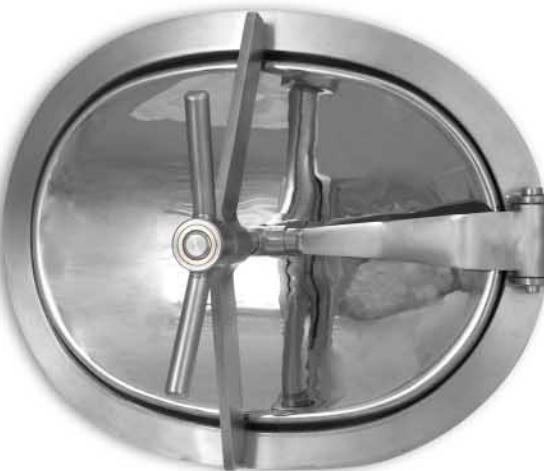
Oval shaped manhole door type "fruit juice" in AISI 304 or AISI 316 stainless steel - inward opening - frame fabricated in flat stainless steel - access 445 x 340 mm (available on request with bending for various vat diameters).
