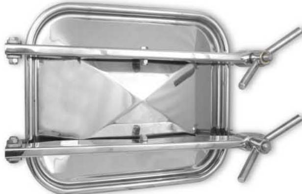
Rectangular manhole door for winemakers in AISI 304 or AISI 316 stainless steel - frame in flat stainless steel or iron - horizontal outward opening - access 530 x 410 mm.
