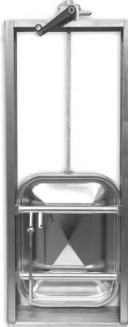
Rectangular manhole door in AISI 304/L or AISI 316/L stainless steel frame in flat stainless steel - vertical guillotine opening - access 530 x 410 mm.
