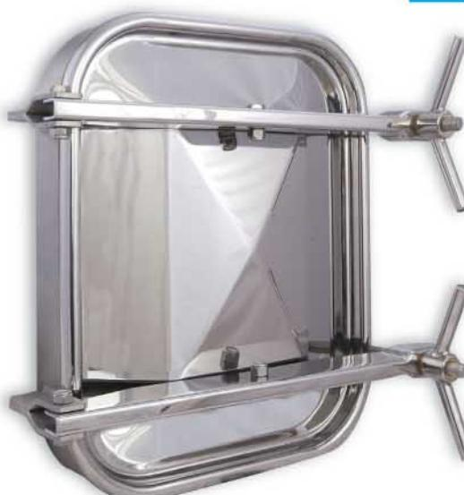
Rectangular manhole door for winemakers in AISI 304 or AISI 316 stainless steel - frame in flat stainless steel or iron - vertical outward opening access 530 x 410 mm.
