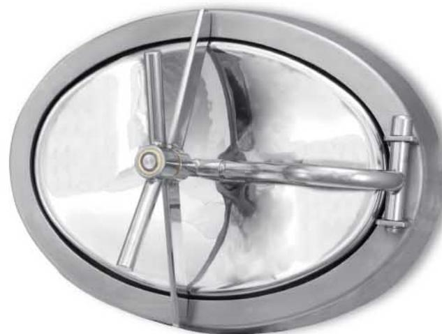
Oval shaped manhole door type "fruit juice" in AISI 304 or AISI 316 stainless steel - inward opening - frame fabricated in flat stainless steel 30 x 12 mm. H 80x3 mm. - access 440 x 310 mm.
